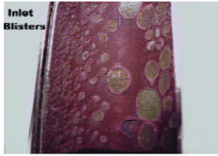
Fig. 7A: Blisters (note white salts)
