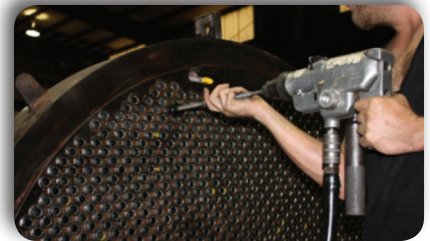
Alloy tube end inserts for hot, acidic service
