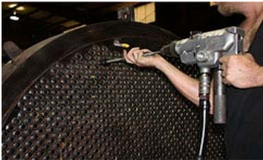
Curran provides hydraulically expanded tube sleeves and full length liners.
