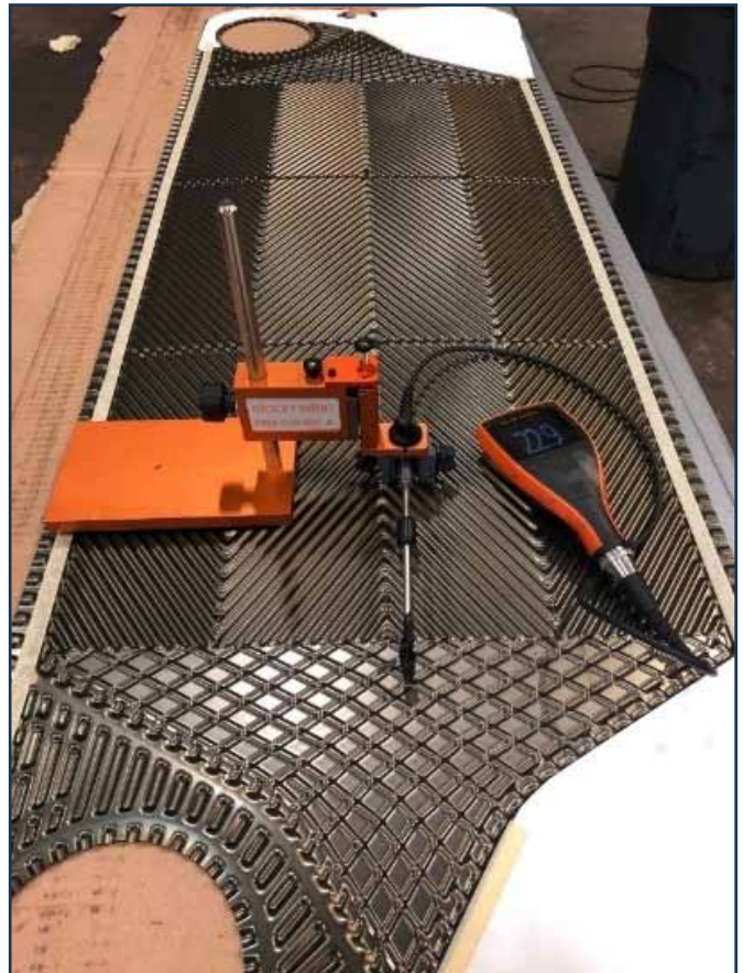
Exchanger plate with Curramix release coating applied to 23 microns total thickness.
