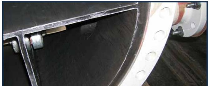
New fabrication heat exchanger channel, ID coated with Curran 1500, applied to 0.040" in a single coat.
