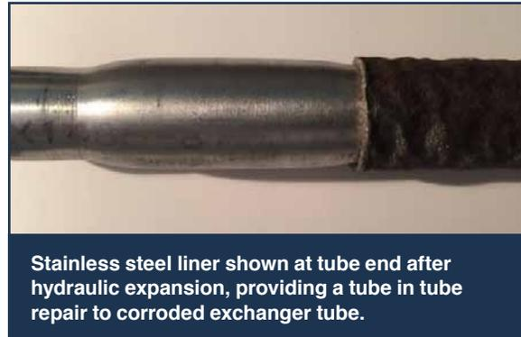
**Stainless steel liner shown at tube end after hydraulic expansion, providing a tube in tube repair to corroded exchanger tube.**
