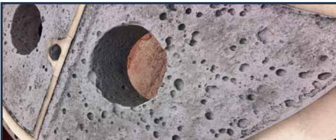
Channel in cooling water, pitted surface blasted clean exposing many pits deeper than 0.0625"
