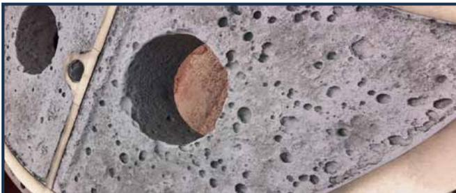
Channel in cooling water, pitted surface blasted clean exposing many pits deeper than 0.0625"
