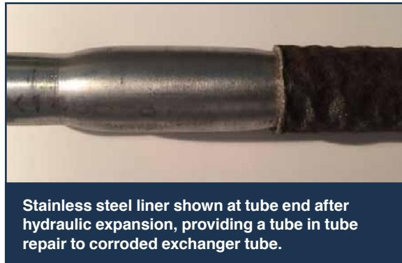
**Stainless steel liner shown at tube end after hydraulic expansion, providing a tube in tube repair to corroded exchanger tube.**
