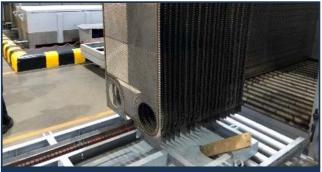
Coated plates being loaded in to oven for low temperature cure.
