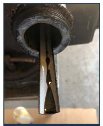
Curramix 3500, 60-days static soak in test fixture at 650F; crude oil flowing down coated tube.
