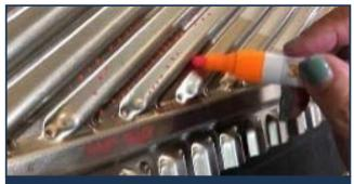
Dyne pen 30 ink test; ink will not wet out on surfaces with lower than 30 dynes/cm2 surface energy. Image shows ink as droplets at coating substrate, and a continuous film at uncoated area.
