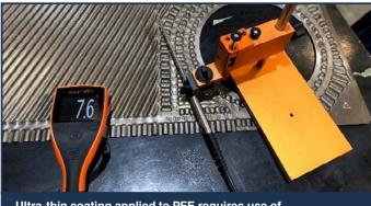
Ultra-thin coating applied to PFE requires use of positioning jig to record precise film thickness measurements, instrument shows 7.6 microns thickness.
