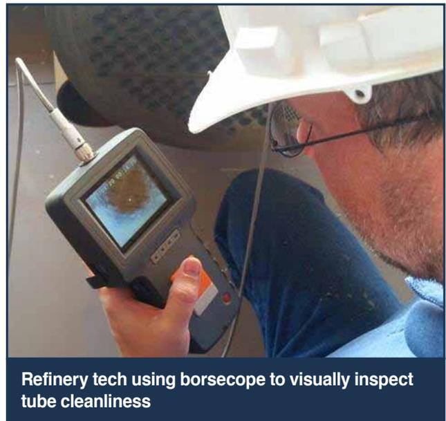
Refinery tech using borescope to visually inspect tube cleanliness
