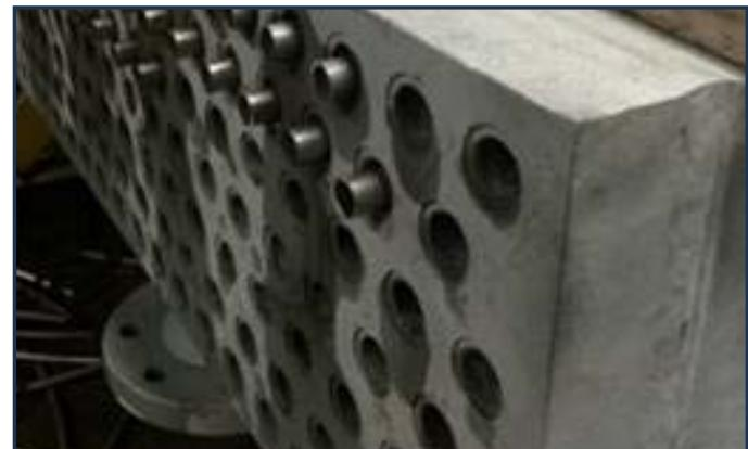
Full-length alloy liners used in a new fabrication replacement air cooler; client upgraded only primary inlet section where operating history showed tube corrosion was severe.
