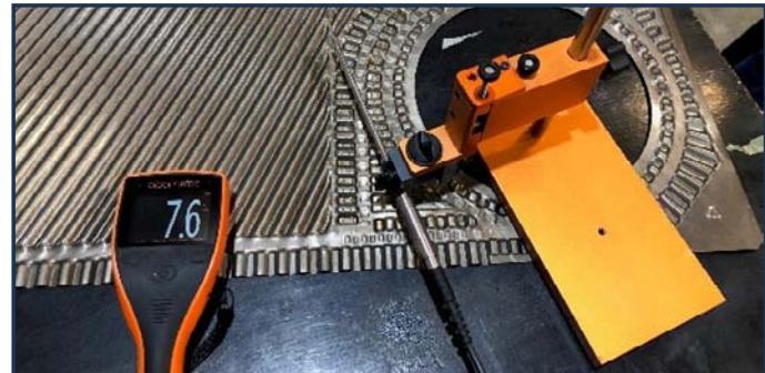
**Ultra-thin Curran coating applied to PFE requires use of positioning jig to record precise film thickness measurements, instrument shows 7.6 microns thickness.**
