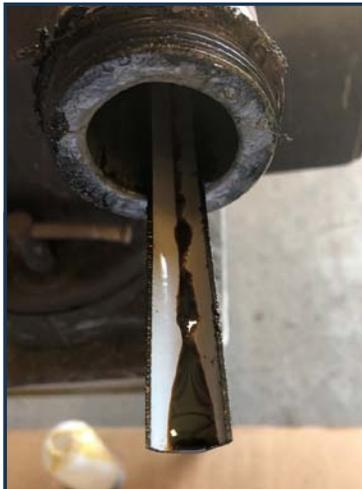
**Curramix 3500 – 60 days static soak in test fixture at 650F; crude oil flowing down coated tube.**
