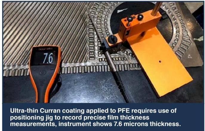
**Ultra-thin Curran coating applied to PFE requires use of positioning jig to record precise film thickness measurements, instrument shows 7.6 microns thickness.**
