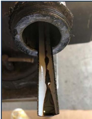
**Curramix 3500 – 60 days static soak in test fixture at 650°F; crude oil flowing down coated tube.**
