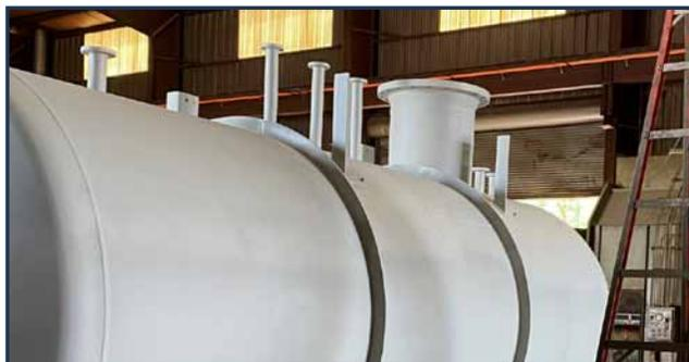
7' diameter vessel in H2S storage service; internally coated with Advanced Polymers/Chepline; externally coated with Hempatop Repel 800 system.
