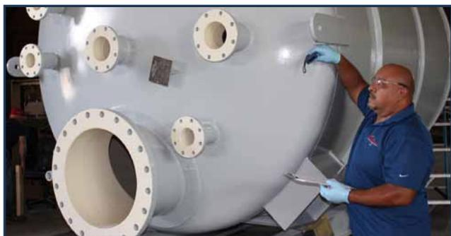
"Boil down" vessel internally coated with Curran 1200 novolac epoxy, externally painted with Carboline IOZ, epoxy and urethane system.
