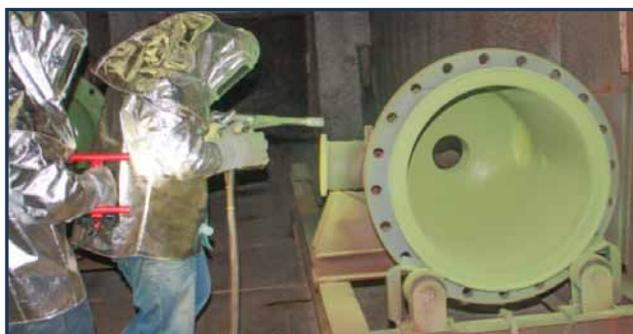
Curran coating tech using hot flock method to apply Chemours ETFE fluoropolymer to vessel head; coating is catalyzed at 625F.
