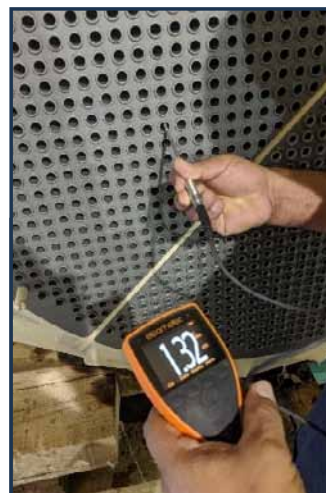
Gauge shows coating thickness, .00132” down tube.
