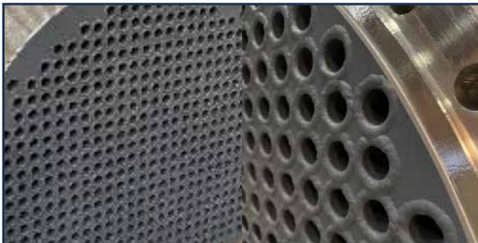
Duplex SS tube bundle coated with Curramic 3500™, a ceramic low-surface energy release coating applied at 30 microns total DFT.
