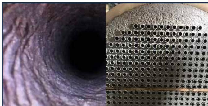
(Figure 2) Uncoated exchanger and tubesheet, after Curran cleaned for IRIS NDE.
