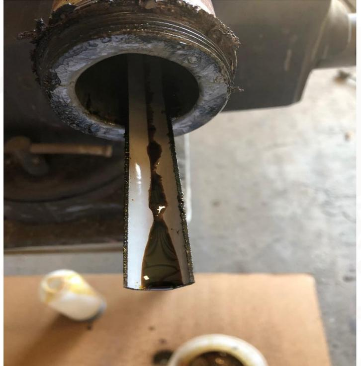
**Curramix 3500 non-stick benefits after static soak in hot crude; (below) image of coated ID and uncoated OD subjected to high chloride well water.**
